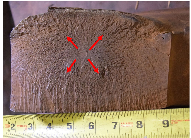
Figure 20. Fractured alloy steel grate rib showing fracture features. Arrows indicate overload fracture initiation site.
