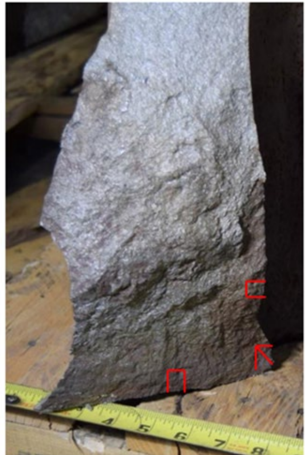
Figure 14. Sample locations used for microstructure examination. In-service fracture is slightly discolored compared to laboratory fracture to expose the crack.
