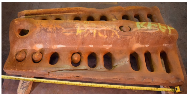
Figure 19. As received casting for failure analysis.
