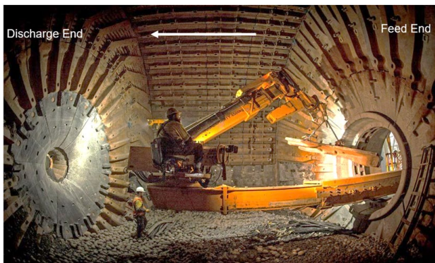
Figure 2. An example of alloy steel liners used in a SAG mill. (Artwork courtesy of ME Global.)
