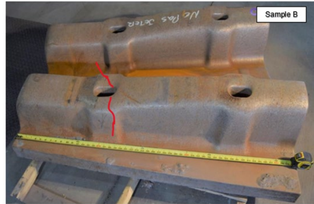
Figure 13. Image of white iron casting where fracture occurred. Casting had to be broken open to expose the fracture face.
