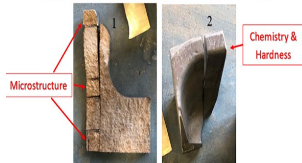
Figure 10. Sectioning and locations for chemistry, hardness and microstructure analysis.
